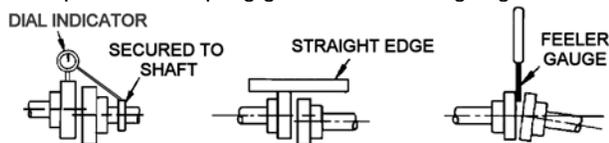
Figure 5 – Coupling Alignment
