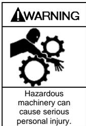
Failure to disconnect and lockout electrical power or engine drive before attempting maintenance can cause severe personal injury or death
