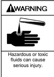
**If pumping hazardous or toxic fluids, system must be flushed prior to performing service**
