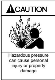
**Pumps operating against a closed valve can cause system failure, personal injury and property damage**
