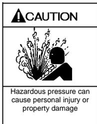
Incorrect settings of the pressure relief valve can cause pump component failure, personal injury, and property damage.
